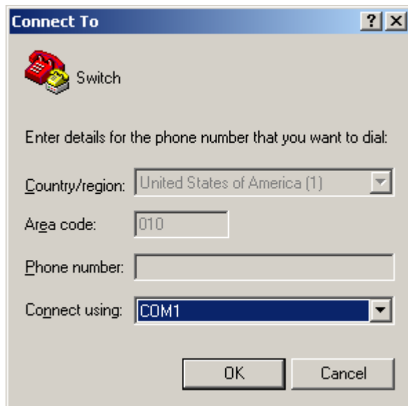
Figure 17 Setting the serial port used by the HyperTerminal connection
